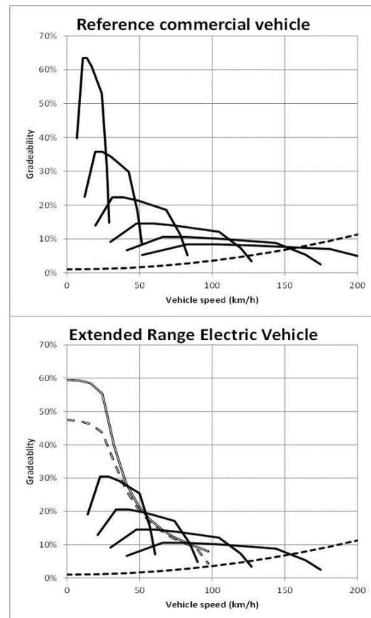
Figure 2. Original and EREV truck tractive force diagrams
