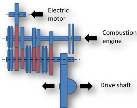
Figure 1. EREV Gearbox layout
