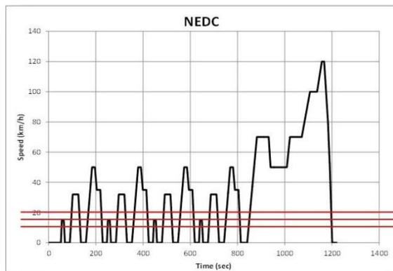
Figure 3. NEDC with three different 1-2 upshift lines
